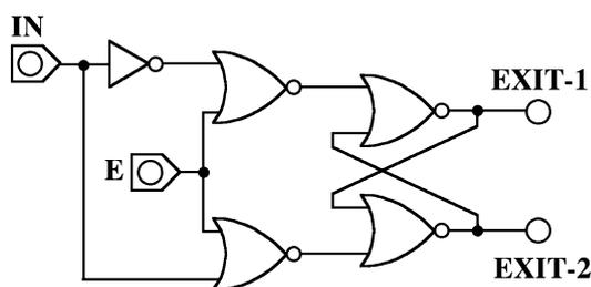
**Scheme 1** The logic scheme of a possible D-latch system. E represents the enabler/disabler input, and IN is the data input.
