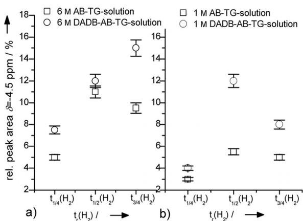
Figure 7. Evolution analysis of the relative areas of the BCDB-related  $^{11}\text{B}$  NMR spectroscopic peak at  $\delta = -4.5$  ppm for different  $[\text{AB}]_0$  values during the dehydrogenation reaction of (a) 6.0 M and (b) 1.0 M solutions of AB/TG and AB/DADB/TG mixtures. The addition of DADB significantly promotes the formation of BCDB.
