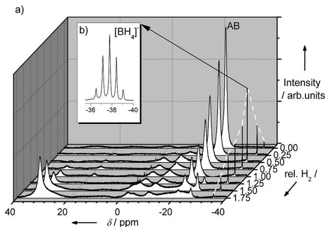
Figure 4. (a) <sup>11</sup>B{<sup>1</sup>H} NMR spectra depicting the dehydrogenation evolution form an AB/TG solution ([AB]<sub>0</sub> = 6.0 M) at 70 °C. (b) The quintet signal at  $\delta \approx (-36.5 \pm 0.5)$  ppm in the coupled spectra is identified as the BH<sub>4</sub> resonance of DADB and can be traced almost along the whole dehydrogenation process.
