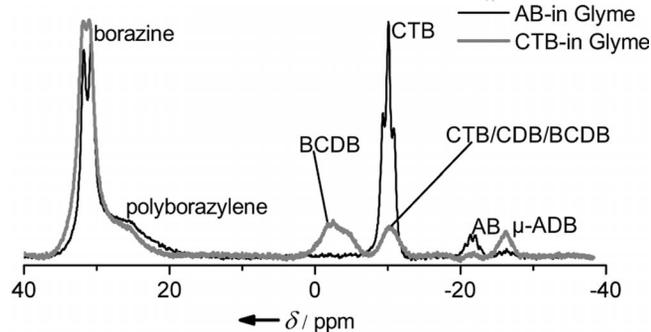
Figure 8. Coupled  $^{11}\text{B}\{^1\text{H}\}$  NMR spectra<sup>[8]</sup> of samples of AB (black line) and CTB (grey line) in glyme, which were dehydrogenated at 90 and 130 °C for 4 h, respectively. The spectrum of CTB does not show any signal of BCDB or CDB, whereas highly concentrated AB/TG solutions react to form CDB, BCDB and significant amounts of  $\mu\text{-ADB}$ .
