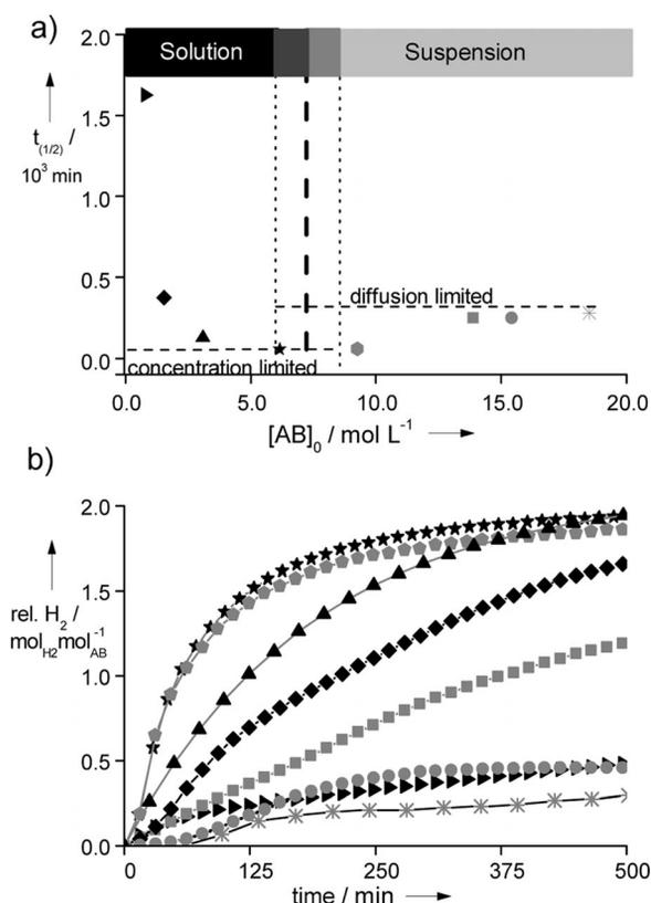
Figure 1. Hydrogen-release characteristics of AB in TG at  $T = 70\text{ }^{\circ}\text{C}$  for mixtures with concentrations between 1.5 and 18 M. (a) Plot of the half-time of the total hydrogen release (i.e., the equivalent of 1 mol of  $\text{H}_2$  per mol of  $\text{BH}_3\text{NH}_3$ ) versus the concentration of the initial AB concentration in TG. (b) Amount of hydrogen released as a function of time given in mol  $\text{H}_2$  per mol  $\text{BH}_3\text{NH}_3$ .
