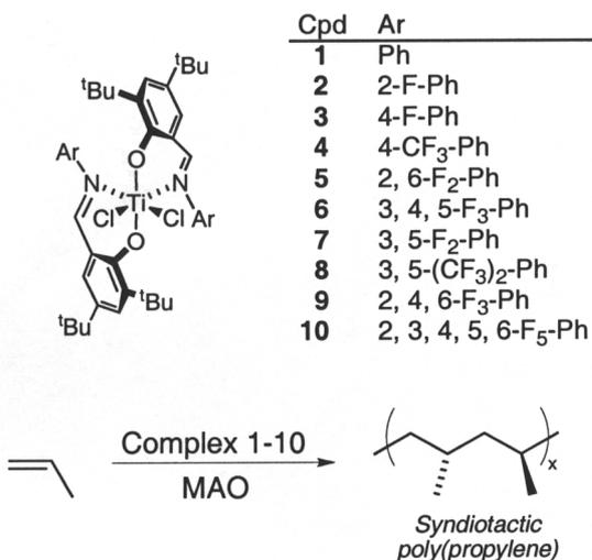
Scheme 1. Catalysts for syndiospecific propylene polymerization.
