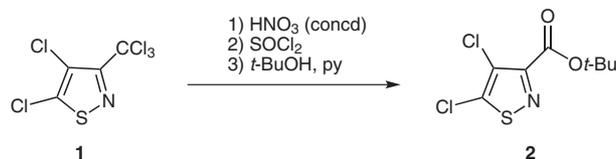
**Scheme 1** Preparation of *tert*-butyl 4,5-dichloroisothiazole-3-carboxylate (**2**)
