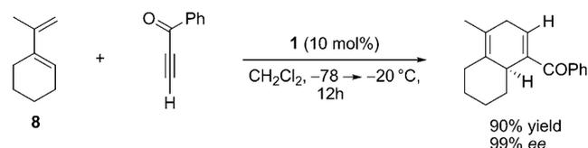
**Scheme 2.** Diels–Alder reaction of an acetylenic ketone without a terminal silyl group.
