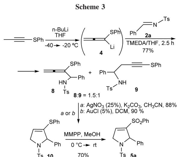
$\text{AuCl}$  catalysis afforded the corresponding 3-phenylthio-3-pyrroline **10**, which by oxidation with MMPP was converted into sulfone **5a**. When the transformation was carried out in a single step by reaction of **2a** with **6**<sup>12,19</sup> in the presence of a nucleophilic mediator, regioisomeric 2-aryl-4-(phenylsulfonyl)-1-tosyl-3-pyrroline **7a** was obtained.
