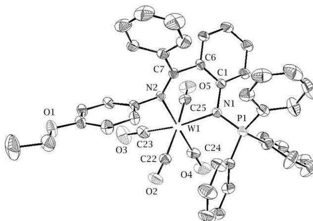
**Fig. 1** Molecular structure of **3** (depicted with 35% probability ellipsoids, H atoms are omitted for clarity). Selected bond distances (Å) and angles (°): P(1)-N(1) = 1.606(5); N(1)-W(1) = 2.260(4); N(2)-W(1) = 2.260(4); C(23)-W(1) = 1.944(7); C(24)-W(1) = 1.952(6); N(2)-W(1)-N(1) = 76.21(16); N(1)-W(1)-C(23) = 171.3(2); N(2)-W(1)-C(24) = 173.5(2); C(23)-W(1)-C(24) = 87.6(3).
