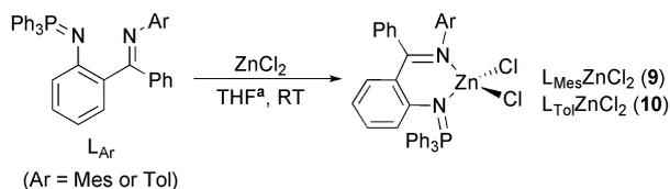
**Scheme 4** In reactions with  $L_{Mes}$  a saturated solution is required to form **10**
