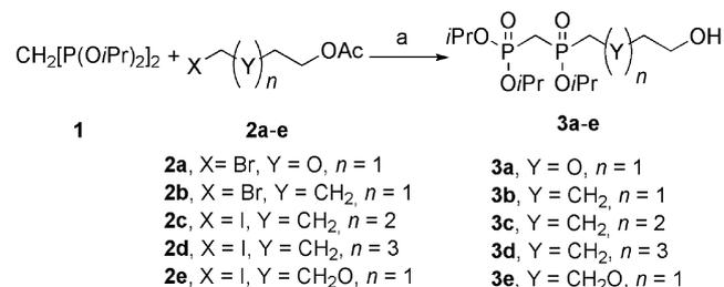
Scheme 1. Arbuzov reaction of **1** with alkyl halides **2a–e**. Reagents and conditions: a) 1. 120 °C, 2. DMSO, 3. HCl, EtOH.
