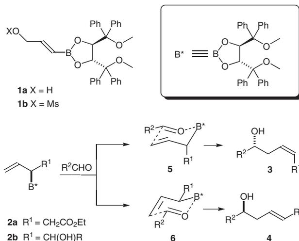
**Scheme 1** Transition structures for the allyl addition of  $\alpha$ -substituted allylboronates **2** to aldehydes
