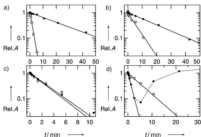
**Figure 5.** Changes in the absorbance maxima during irradiation of *trans*-**1** (a), *cis*-**1** (b), (*E*)-**2** (c), and (*Z*)-**2** (d) at 80 K in 2-methylpentane glass and 273 K in 2-methylpentane solution. The closed and open circles represent absorbance changes at 80 and 273 K, respectively.
