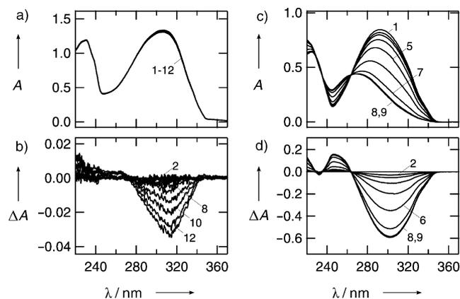
**Figure 1.** Progress of the photoreaction ( $\lambda > 280$  nm) of *trans*-1 at 80 K in 2-methylpentane glass (a and c) and in 2-methylpentane solvent at 273 K (b and d). Changes in the absorption spectra versus time (0, 5, 10, 20, 40, 80, 160, 320, 640, 1280, 2560, and 5120 s for a; the same intervals to 640 s for b) and difference absorption bands ( $A_t - A_0$ ) for the 80 K (c) and 273 K (d) data are shown.
