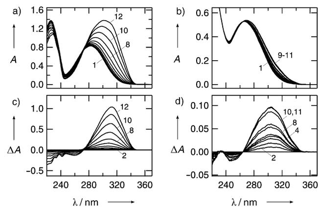
**Figure 2.** Progress of the photoreaction ( $\lambda > 280$  nm) of *cis*-1 at 80 K in 2-methylpentane glass (a and c) and in 2-methylpentane solvent at 273 K (b and d). Changes in the absorption curves versus time (0, 5, 10, 20, 40, 80, 160, 320, 640, 1280, 2560, and 5120 s for a; same intervals to 2560 s for b) and difference absorption bands ( $A_t - A_0$ ) for the 80 K (c) and 273 K (d) data are shown.
