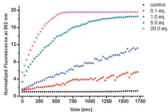
**Fig. 3** Kinetics of fluorescence over background at varying  $\text{Cu}^{2+}$  levels. Conditions:  $[\mathbf{1}] = 1.0 \times 10^{-6}$  M,  $\lambda_{\text{ex}} = 450$  nm, buffer pH = 5.0.
