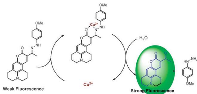
**Scheme 2**  $\text{Cu}^{2+}$ -induced catalytic sensing cycle of **1**.
