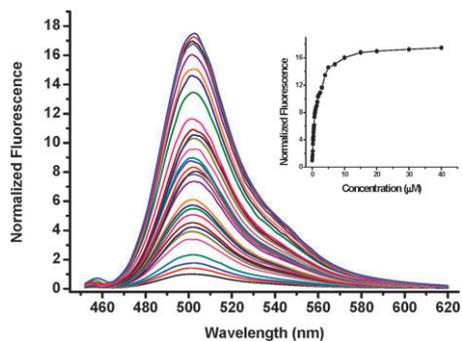
**Fig. 1** Fluorescence emission spectra obtained by addition of  $\text{Cu}^{2+}$  (0–40  $\mu\text{M}$ ) to pH 5.0 buffer solution (acetonitrile : 0.01 M acetate buffer = 5 : 5) containing **1** (1  $\mu\text{M}$ ). Inset: plot of normalized fluorescence intensities of **1** at 502 nm versus  $\text{Cu}^{2+}$  concentration.
