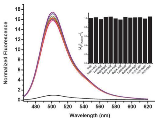
**Fig. 4** Fluorescence emission spectra obtained by addition of  $\text{Cu}^{2+}$  ( $10 \mu\text{M}$ ) to pH 5.0 buffer solution (acetonitrile : 0.01 M acetate buffer = 5 : 5) containing **1** ( $1 \mu\text{M}$ ) and metal ions ( $100 \mu\text{M}$ ). Inset: fluorescence intensities of **1** ( $1 \mu\text{M}$ ) in the presence of  $\text{Cu}^{2+}$  ( $10 \mu\text{M}$ ) and metal ions ( $100 \mu\text{M}$ ).
