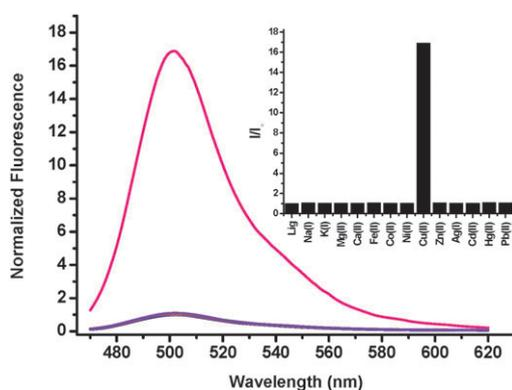
**Fig. 2** Fluorescence emission spectra obtained by addition of various metal ions to pH 5.0 buffer solution (acetonitrile : 0.01 M acetate buffer = 5 : 5) containing **1** (1  $\mu\text{M}$ ). Inset: plot of normalized fluorescence intensities of **1** at 502 nm versus metal ions.
