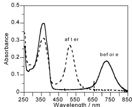
**Figure 4.** Absorption spectra of a glassy film of **1** containing 2 wt % of **d-12** before and after photoirradiation, respectively. The photoirradiation was performed with a 366-nm light source at 90 °C.
