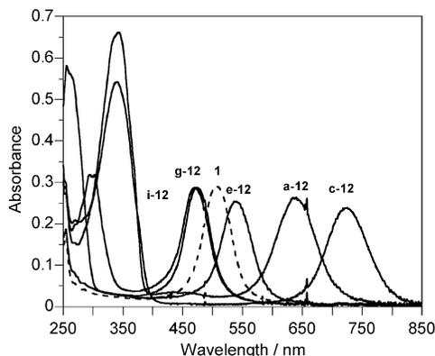
**Figure 2.** Absorption spectra of the glassy films of pure **1** and **1** containing 2 wt % of **a-12**, **c-12**, **e-12**, **g-12**, and **i-12**, respectively. The films were quenched from 90 °C, and their thickness was controlled by a 5- $\mu$ m spherical silica spacer.
