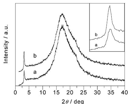
**Figure 9.** X-ray diffraction patterns for pure **1** (a) and **1** containing 2 wt % of **a-11** (b) at 90 °C. Inset is the magnification of the small angle peaks.
