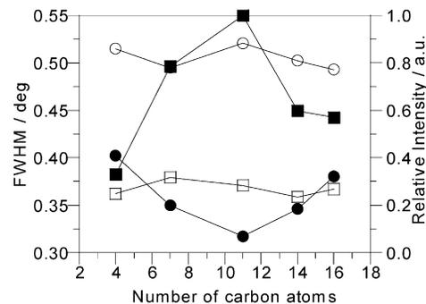
**Figure 10.** Effect of the alkyl chain length on the half-width (circles) and the relative intensity (squares) of the small-angle X-ray diffraction peaks for **1** containing 2 wt % of **a-n** at 90 °C (closed markers) and 110 °C (open markers). The lines are visual guides.
