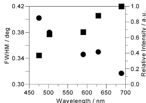
**Figure 11.** Relation between the wavelength of maximum reflections and the parameters (half-width, circles; and relative intensity, squares) of small-angle X-ray diffraction peaks for **1** containing 2 wt % of **a-n** at 90 °C. These data are extracted from the results of Figures 5 and 6.
