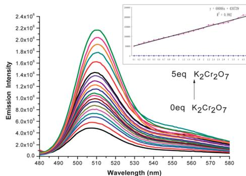
Fig. 2 The fluorescence spectra of **1** (10  $\mu$ M) upon addition of  $Cr_2O_7^{2-}$  (0, 0.1, 0.2, 0.3, 0.4, 0.5, 0.6, 0.7, 0.8, 0.9, 1.0, 1.2, 1.5, 2.0, 2.5, 3.0, 3.5, 4.0, 4.5, 5.0 equiv.,  $K_2Cr_2O_7$ ) in  $H_2O : DMF = 3 : 7$ . Inset: the linear relationship of fluorescence titration.
