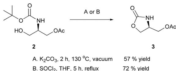
**Scheme 3.** Synthesis of enantiomerically enriched 4-acetoxymethyl-2-oxazolidinone.
