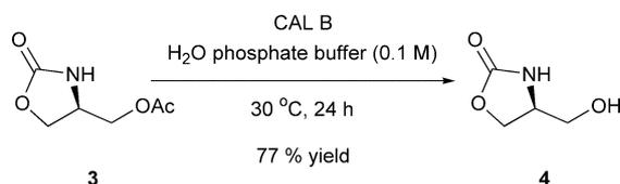
**Scheme 4.** Hydrolysis of 4-acetoxymethyl-2-oxazolidinone.
