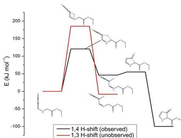
**Figure 1** Energy surface for pyrrolone formation and (in red) imidoylketene formation (cf. Scheme 1,  $R^2 = \text{CO}_2\text{Et}$ )
