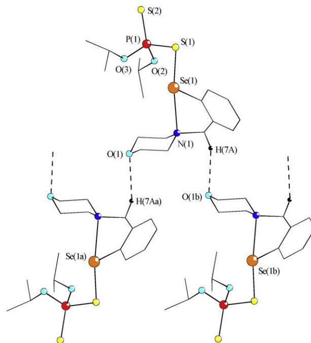
**Fig. 5.** View of the chain polymer based on sulfur–hydrogen contacts between S isomers in the crystal of **6** [only hydrogens involved in intermolecular contacts are shown; symmetry equivalent atoms (–0.5 + x, 0.5 – y, 2 – z) and (0.5 + x, 0.5 – y, 2 – z) are given by “a” and “b”, respectively].
