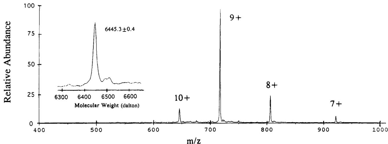
**Figure 2.** Mass spectrum of the peak eluting at 15 min produced by the reaction of Noba with p7 (Figure 1c).
