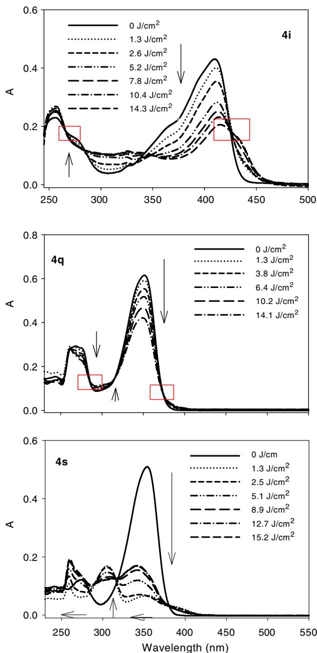
**Figure 1.** Photodegradation of pyrrolo[3,4-*h*]quinolin-2-ones. Absorption spectra of compound **4i** (upper panel), **4q** (middle panel) and **4s** (lower panel) at the concentration of 20  $\mu\text{M}$  in DMSO were recorded after exposure to increasing UV-A doses. Red squares in the graphs indicate the presence of isosbestic points.
