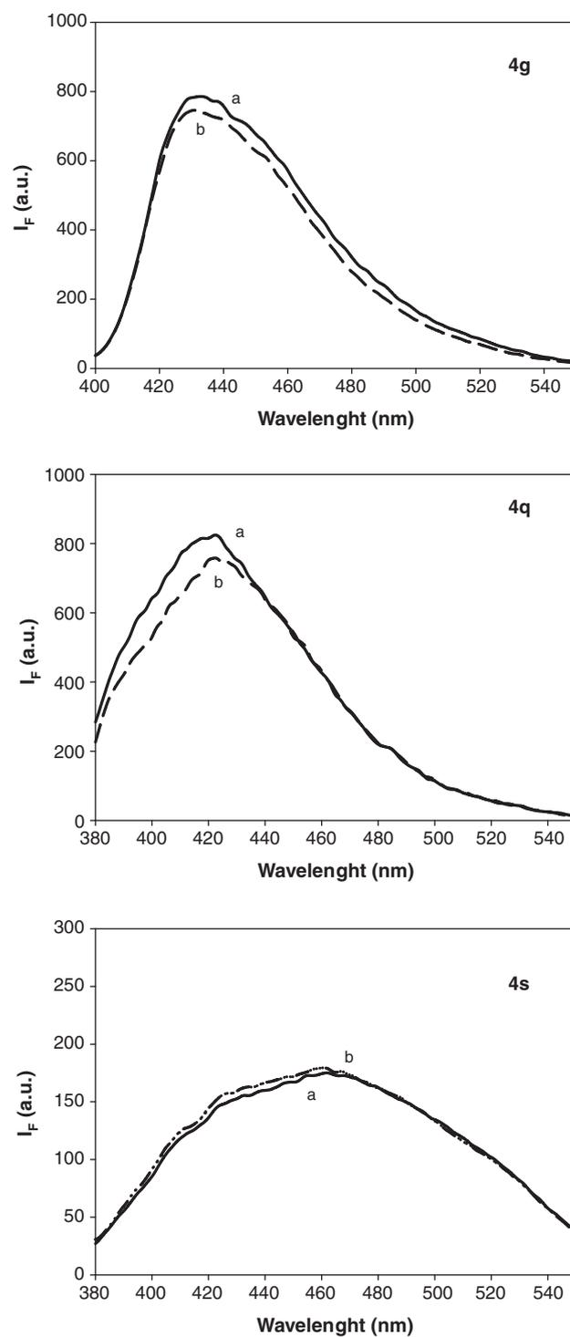
**Figure 7.** Fluorimetric titrations of stDNA ( $a = 0 \mu\text{M}$ ;  $b = 100 \mu\text{M}$ ) to compounds **4g**, **4q**, and **4s** at a ligand concentration of 10  $\mu\text{M}$ .
