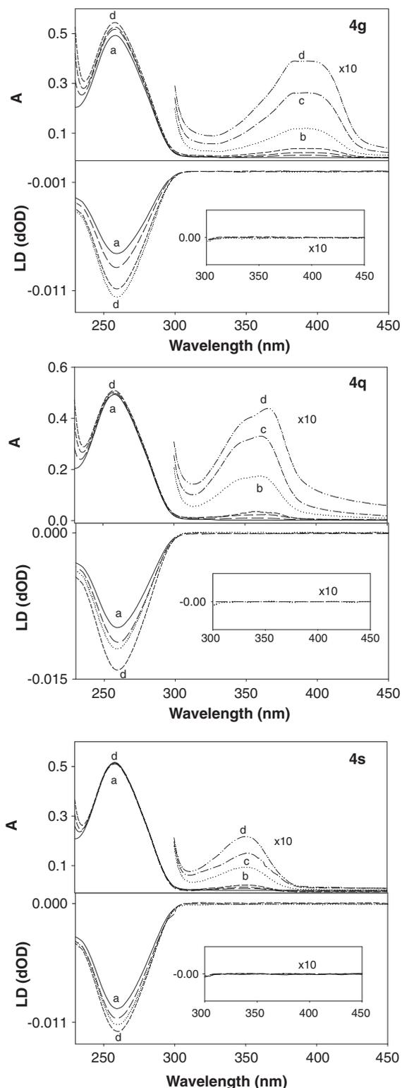
**Figure 6.** Absorbance (A) and linear dichroism (LD) spectra of mixtures of st-DNA and **4g** and **4q** (upper panels) and **4s** (lower panel) at different [drug]/[DNA] ratios ( $a = 0$ ;  $b = 0.01$ ;  $c = 0.02$ ;  $d = 0.03$ ) in phosphate buffer 10 mM, pH 7.2.
