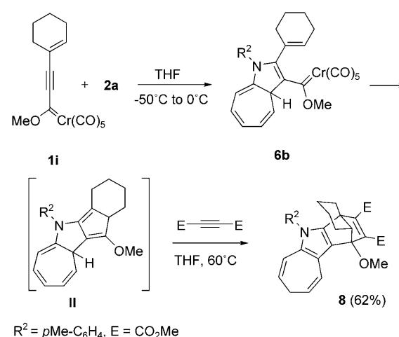
Scheme 6. Formation and Diels–Alder reaction of the cyclopentannulation intermediate **II** with dimethyl acetylenedicarboxylate.
