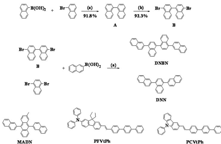
**Scheme 1.** Synthetic route for new host materials and the structures of the dopant materials. (a) toluene/ethanol, Na<sub>2</sub>CO<sub>3</sub> (2M), Pd(PPh<sub>3</sub>)<sub>4</sub>, reflux, 4h. (b) Br<sub>2</sub>/CH<sub>2</sub>Cl<sub>2</sub>, rt, 2 h.
