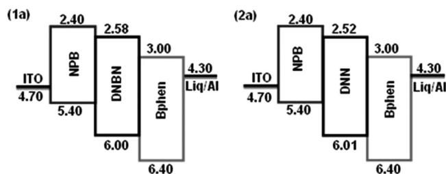
**Figure 2.** Energy diagrams of non-doped devices **1a-2c**.
