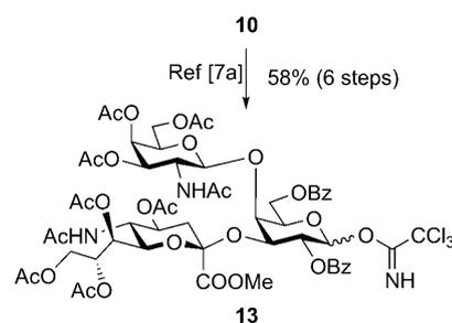
Scheme 3. Synthesis of the GM2-core donor **13**. a) i) Zn, AcOH/MeOH (1:1), RT; ii) Ac<sub>2</sub>O/Pyr, RT, 81%; b) i) H<sub>2</sub>, Pd(OH)<sub>2</sub>-C/1,4-dioxane, RT; ii) Bz<sub>2</sub>O, DMAP/Pyr, RT, 95%; c) i) CAN, MeCN/PhMe/H<sub>2</sub>O (6:5:3), RT; ii) CCl<sub>3</sub>CN, DBU/CH<sub>2</sub>Cl<sub>2</sub>, RT, 75%. Bz = benzoyl, CAN = cerium(IV) ammonium nitrate.
