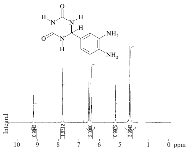
Fig. 1. ^1\text{H} NMR spectrum of 1,2,3,4,5,6-hexahydro-6-(3,4-diaminophenyl)-1,3,5-triazine-2,4-dione (X).
