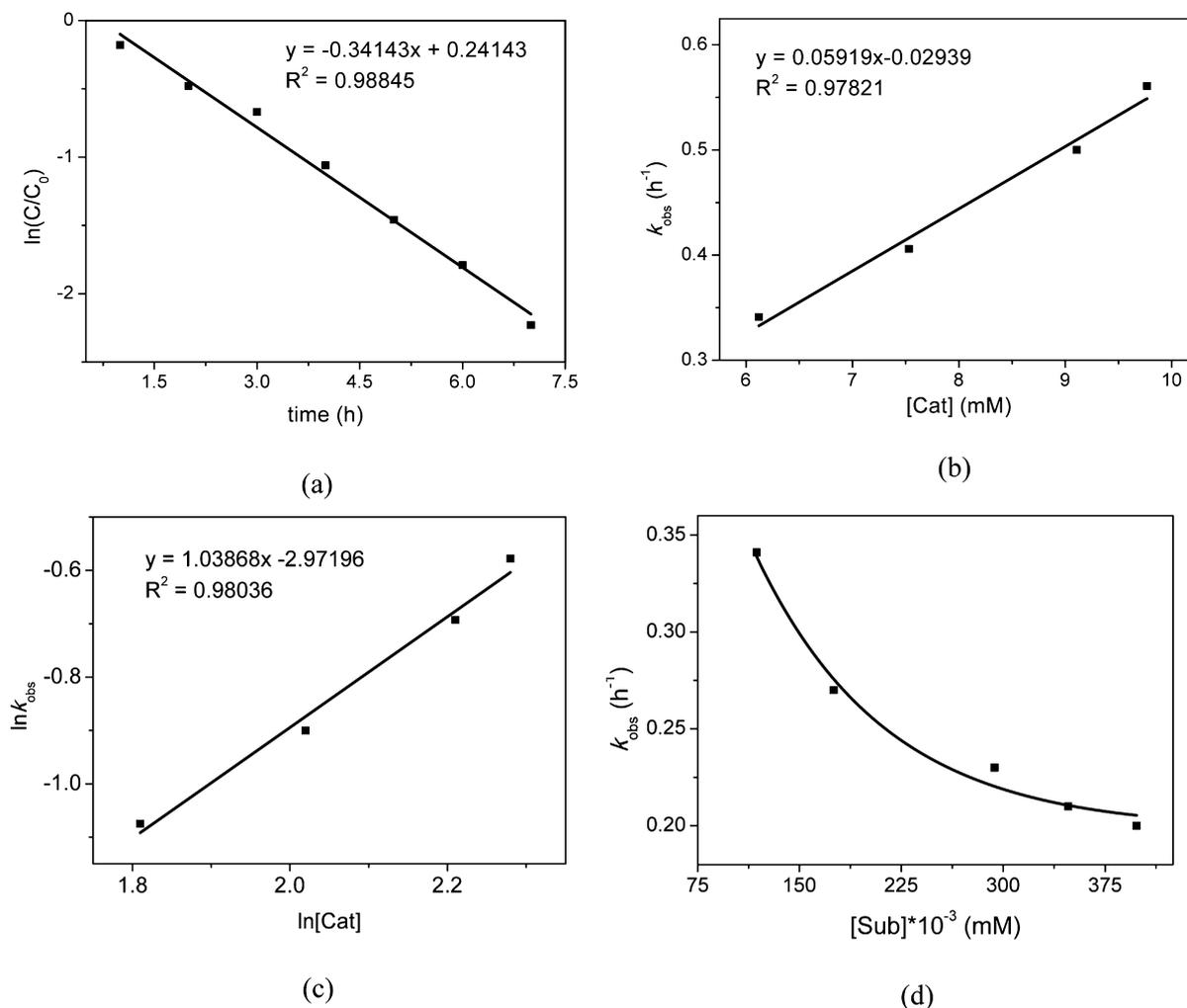
**Figure 3.** Kinetic studies of primary aminoalkene cyclization process monitored by  $^1\text{H}$  NMR spectroscopy in  $\text{C}_6\text{D}_6$ : (a) plot of  $\ln(C/C_0)$  versus time for the cyclization of **3**; (b) plot of  $k_{\text{obs}}$  versus  $[\text{Cat}]$  for the cyclization of **3**; (c) van't Hoff plot of  $\ln k_{\text{obs}}$  versus  $\ln[\text{Cat}]$ ; (d) plot of  $k_{\text{obs}}$  versus  $[\text{Sub}]$  for the cyclization of **3** using catalyst **2**.
