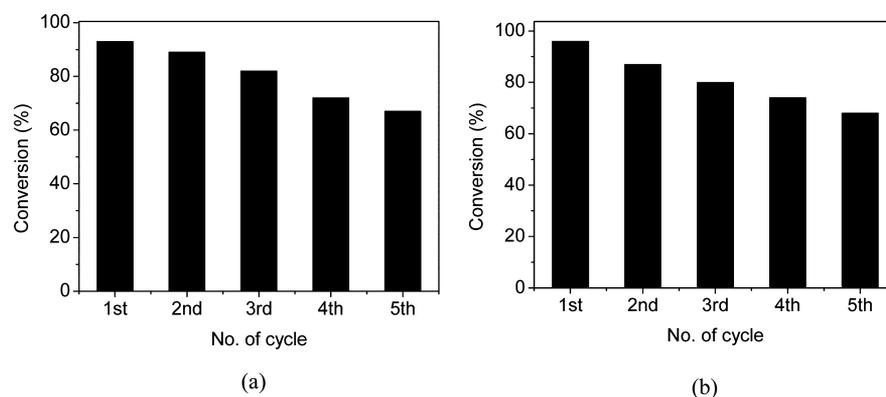
**Figure 7.** Catalyst longevity test for the cyclization of (a) (1-allylcyclohexyl)methylamine (**3**) with catalyst **2** in C<sub>6</sub>D<sub>6</sub> maintaining the reaction bath at 120 °C and (b) benzyl(2,2-diphenyl-4-pentenyl)amine (**10**) with catalyst **2** in C<sub>6</sub>D<sub>6</sub> at 80 °C.
