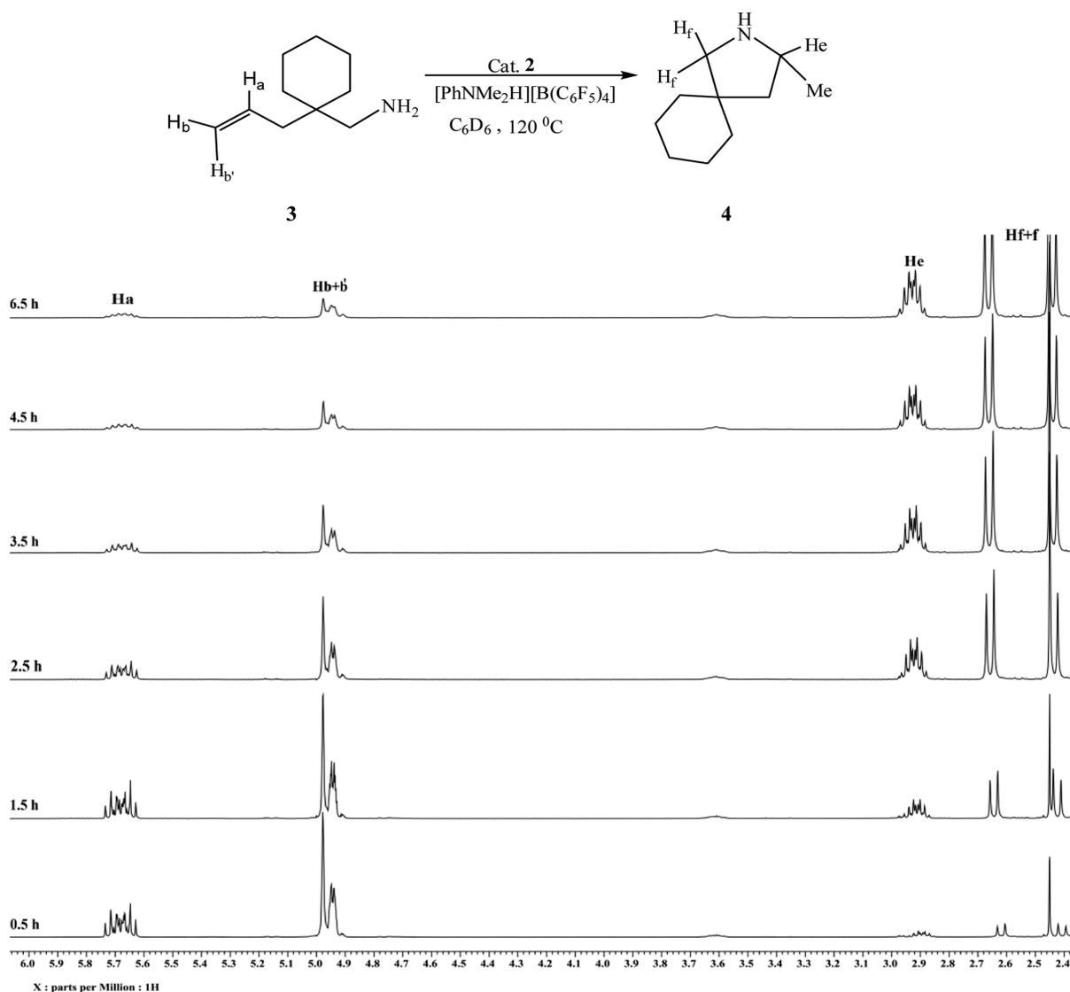
**Figure 2.** Stack plots of  $^1\text{H}$  NMR spectrum for the reaction of (1-allylcyclohexyl)methylamine (**3**) with **2** as catalyst at different time intervals.
