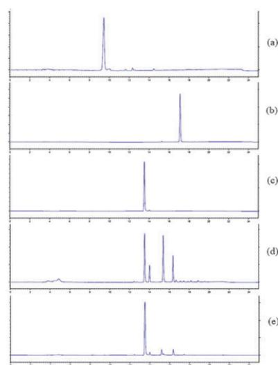
**Fig. 3** HPLC chromatograms of model reaction (C) in the presence of 20 mM Cu(I) in (H<sub>2</sub>O–DMF–*t*-BuOH = 1 : 3 : 1) solution, monitored at 260 nm. (a) pure compound **C-ii**, (namely compound **5**); (b) pure compound **C-i**, namely the alkyne (**i**) in the reaction (C); (c) pure compound **C-iii**, namely the triazole product (**iii**) in the reaction (C); (d) 5 h reaction mixture with Cu(I); (e) 5 h reaction mixture with Cu(I) and fluoride.
