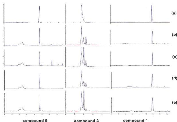
**Fig. 2** HPLC chromatograms of compounds **5**, **3**, and **1** (50 mM for each) in the presence of 20 mM Cu(I) in (H<sub>2</sub>O–DMF–*t*-BuOH = 1 : 3 : 1) solution, monitored at 260 nm. (a) Pure boronic acids; (b) immediately after addition of Cu(I); (c) 5 h after mixing with Cu(I); (d) immediately after addition of Cu(I) and fluoride; (e) 5 h after mixing with Cu(I) and fluoride.
