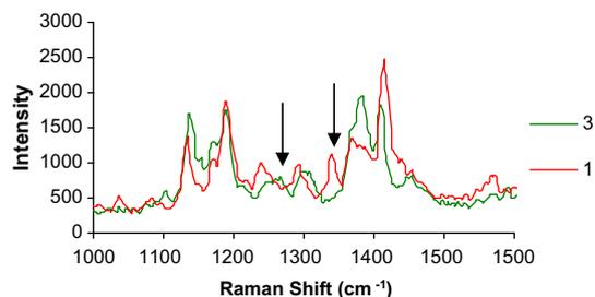
**Figure 2.** Superimposed SERRS spectra for unmasked dyes **1** and **3**. The peaks used for discrimination, at  $1267\text{ cm}^{-1}$  and  $1340\text{ cm}^{-1}$  are highlighted.
