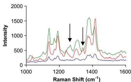
**Figure 3.** SERRS spectra obtained from a mixture of **2** and **4**. (a) without enzyme added (b) with alkaline phosphatase added (c) with  $\beta$ -galactosidase added.
