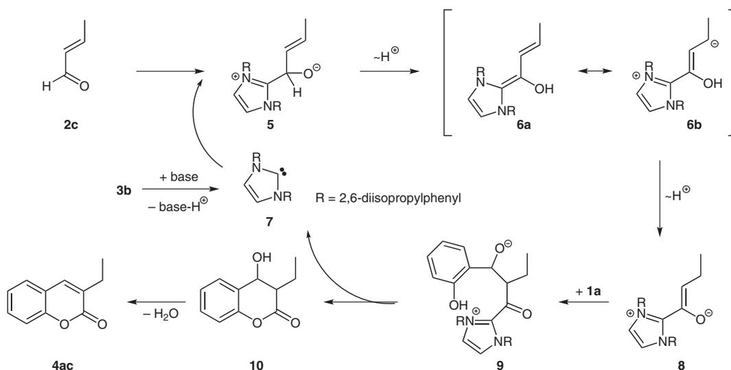
**Scheme 3** Proposed catalytic cycle for the reaction of  $\alpha,\beta$ -unsaturated aldehydes with salicylaldehydes to coumarins
