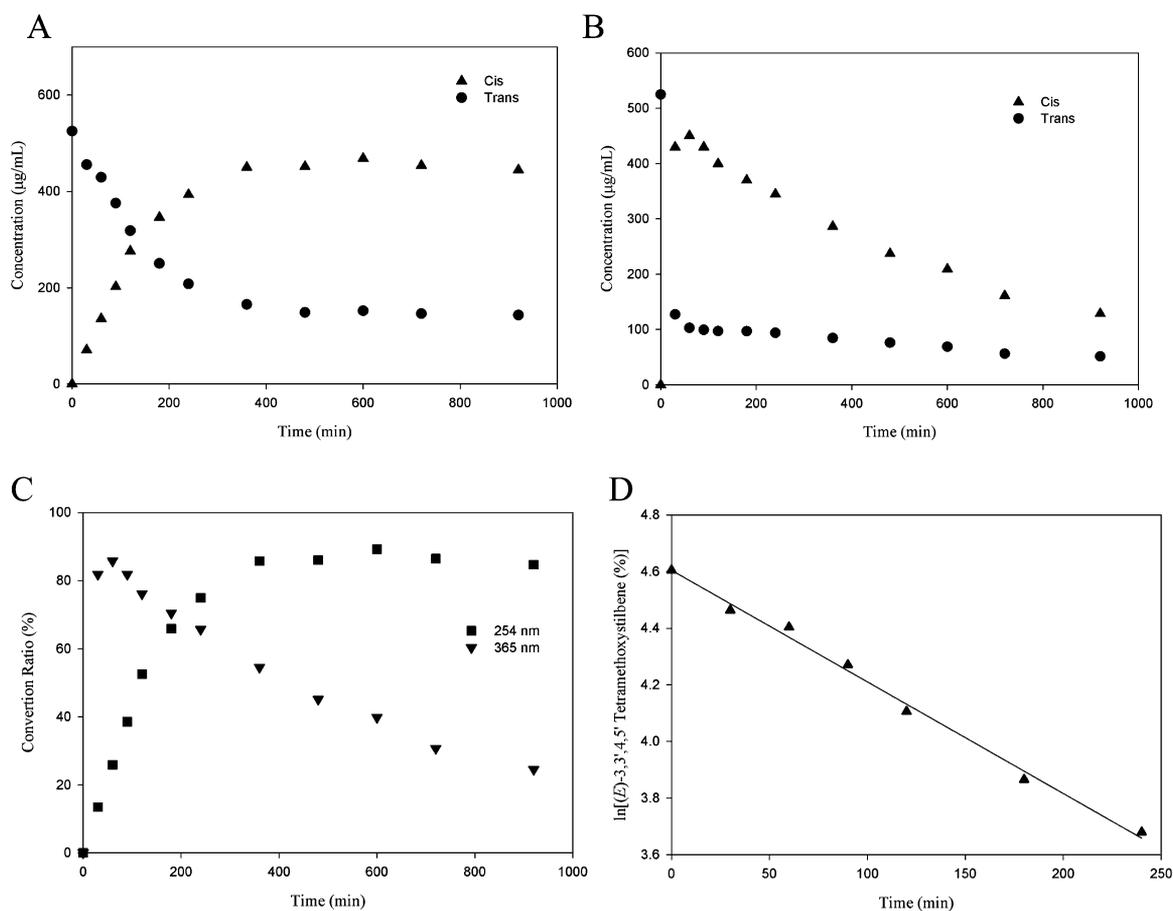
**Figure 2.** Photoisomerization of (E)-2 into (Z)-1 by UV irradiation in tetrahydrofuran (A) at  $\lambda_{254}$  nm and (B) at  $\lambda_{365}$  nm. (C) Assessment of the ratio of (E)-2 into (Z)-1 inversion by UHPLC at  $\lambda_{254}$  nm or  $\lambda_{365}$  nm. (D) Determination of apparent rate constant ( $k_z$ ) and half-life ( $t_{1/2}$ ) of (E)-2 photoisomerization based on pseudo-first-order kinetics by UHPLC.
