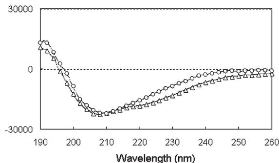
FIGURE 8: Circular dichroism spectra: circle, synthetic monosaccharyl AGH **22**; triangle, synthetic nonglycosylated AGH **23**.
