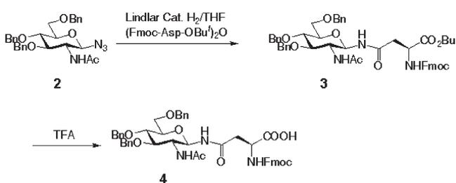
**2** (**10**) was reduced and condensed using an anhydride of Fmoc-Asp-OBu' *in situ* by Matsuo's method (**11**). The Bu' ester was then cleaved with trifluoroacetic acid (TFA) to obtain Fmoc-Asn(GlcNAcBn<sub>3</sub>)-OH **4**.
