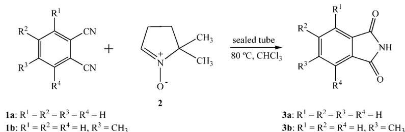
Scheme 1. Synthesis of phthalimides from phthalonitriles and cyclic nitrone.
