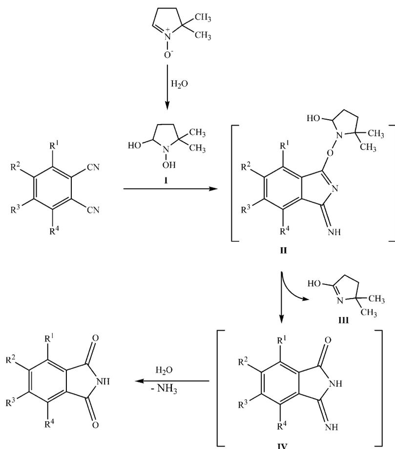
Scheme 2. Proposed mechanism of phthalimide synthesis.
