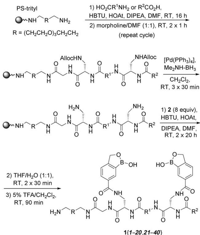
**Scheme 4.** Preparation of library **1{1–20,21–40}**. HBTU = O-(benzotriazol-1-yl)-tetramethyluronium hexafluorophosphate; HOAt = hydroxy-7-azabenzotriazole; DIPEA = diisopropylethylamine; Alloc = allyloxycarbonyl; TFA = trifluoroacetic acid.
