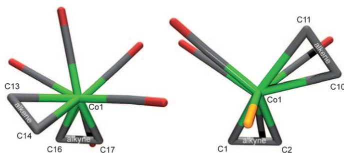
Figure 2. A comparison of the conformation of cobalt complexes **1** (staggered; shown on the left) and **5a** (eclipsed, shown on the right); red = oxygen, orange = phosphorus, grey = carbon, green = cobalt.
