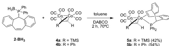
Scheme 3. The reaction of borane-protected **2** (**2-BH<sub>3</sub>**) with acetylene dicobalt complexes.
