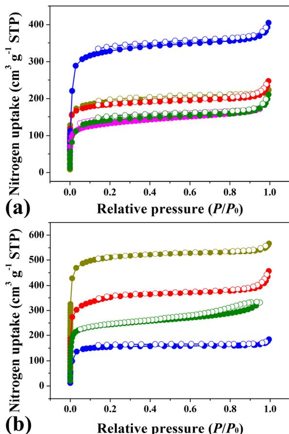
**Figure 3.** (a) The nitrogen isotherms of select PCN-135(L2-n)-type MOFs (dark yellow, L2-1; red, L2-2; blue, L2-9; magenta, L2-17; and olive, L2-22). (b) The nitrogen isotherms of select PCN-135(L4-n)-type MOFs (dark yellow, L4-2; red, L4-3; blue, L4-4; and olive, L4-5). Solid circle, adsorption; and open circle, desorption.
