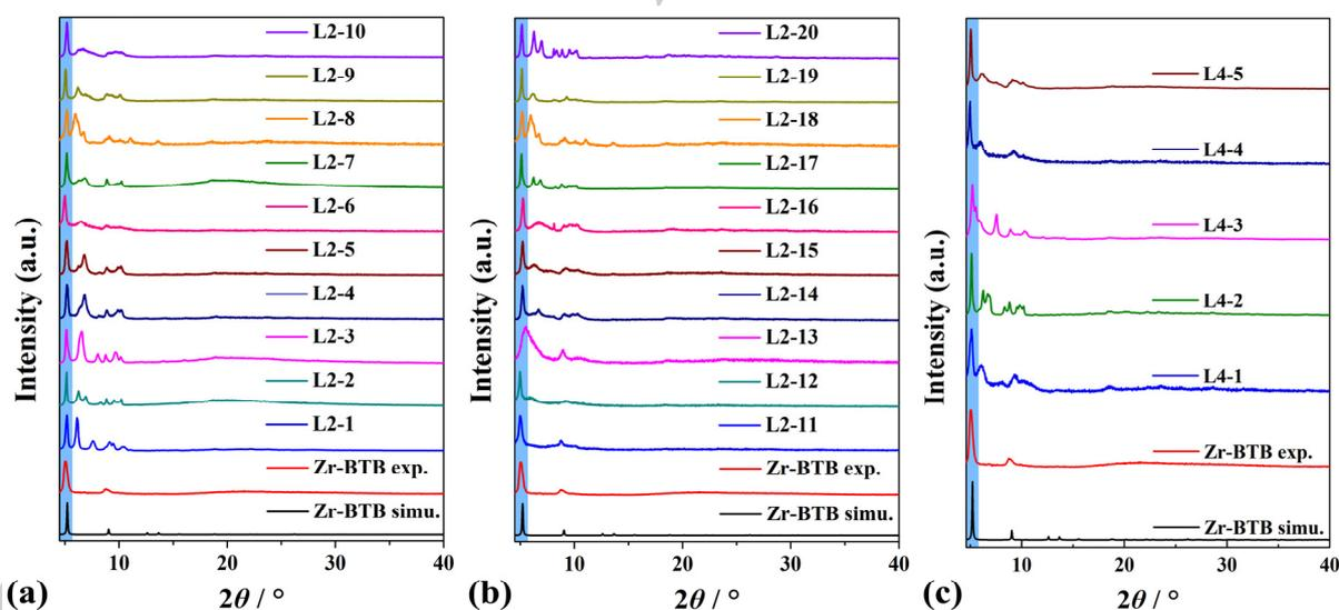
**Figure 2.** The PXRD patterns of the PCN-135 family compared with the experimental and simulated XRD patterns of Zr-BTB. The characteristic peaks of Zr-BTB layer structure and PCN-135 series are highlighted in blue.
