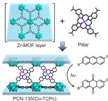
A facile one-pot synthetic strategy was explored to incorporate multi-functionalities into stable zirconium metal-organic layers (MOLs) through the functionalization of  $Zr_6$ -BTB (BTB = benzene-1,3,5-tribenzoate) layers via secondary ligand pillaring. Significantly, a metal-phthalocyanine fragment was successfully incorporated into this Zr-MOL system, giving rise to an ideal platform for the selective oxidation of anthracene.
