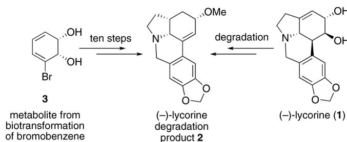
The pentacyclic framework associated with the alkaloid (-)-lycorine (1) can be assembled in as few as six steps from the enantiomerically pure *cis*-1,2-dihydrocatechol 3 which is itself readily available on a large scale through the whole-cell biotransformation of bromobenzene. The methodology has been used in developing the first synthesis of compound 2, a derivative of lycorine.
