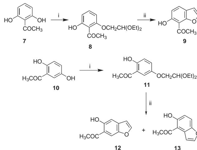
Scheme 2 Reagents and conditions: i)  $\text{BrCH}_2\text{CH}(\text{OEt})_2$ , DMF,  $140^\circ\text{C}$ ; ii) A 15, toluene, reflux.
