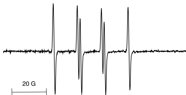
Figure 2. EPR spectrum of reaction mixture containing DMPO, 35 mM, sodium sulfite, 100 mM, and oxidant, K_3Fe(CN)_6 , 3 mM in D_2O , 0.2 mM DTPA, pH_{obs} = 7.1 . Spectrometer settings were as follows: microwave power, 0.625 mW; modulation amplitude, 0.5 G; sweep time, 10.49 s; number of scans, 50. Computer simulation of the spectrum gives the parameters a_N = 14.5 G and a_H = 16.06 G.
