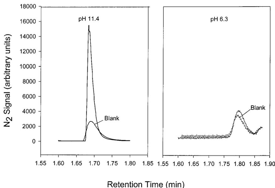
**Figure 2.**  $N_2$  gas chromatograms measured after 240 nm irradiation of 2'-deoxyguanosine for 19 h in 0.02 M  $N_2O$  at pH 11.4 (left panel) and at pH 6.3 (right panel). The left and right panels also contain blank  $N_2$  chromatograms obtained from samples containing 0.02 M  $N_2O$  without dG, irradiated for 19 h at pH 11.4 and 6.3, respectively. The small difference in the  $N_2$  retention times in the two panels is due to a difference in the flow pressure of the He carrier gas.
