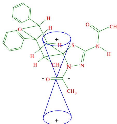
Fig. 10. Anisotropic effect on H-5e and 3-CH<sub>3</sub> protons (+shielding region and -shielding region).
