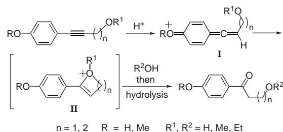
**Scheme 1** Proposed mechanism for the PTSA-catalyzed reaction
