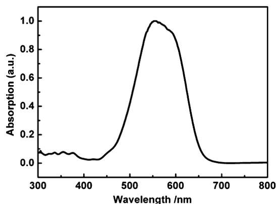
Fig. 2. Absorption spectrum of the spin-coated film.
