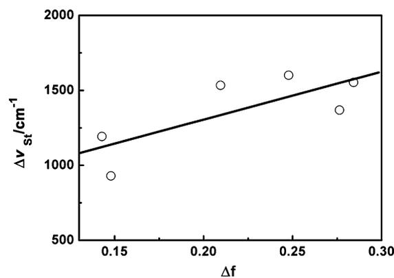
Fig. 5. Plot of Stocks shift  $\Delta v$  of DCDHF-2-V against the solvent polarity function  $\Delta f$ .
