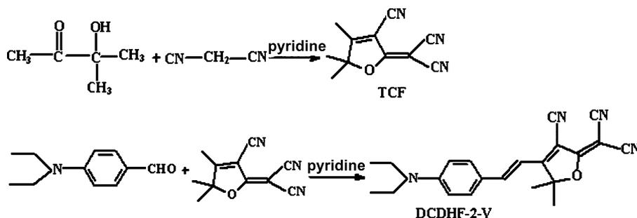
Fig. 1. Synthesis of DCDHF-2-V.
