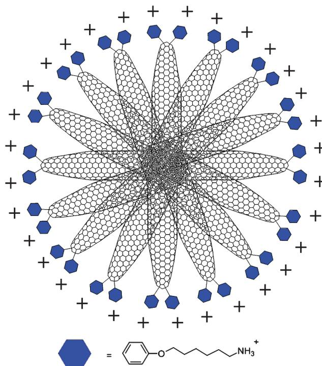
**Fig. 5** *f*-CNHs **11** was prepared from derivative **9** upon treatment with gaseous HCl in DMF (see Experimental). Solubility in water: 0.75 mg/mL.
