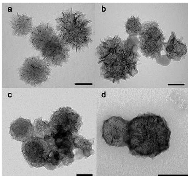
Fig. 2 TEM images of (a) *f*-CNHs 3, (b) *f*-CNHs 4, (c) *f*-CNHs 11, (d) *f*-CNHs 13. Scale bar corresponds to 100 nm.
