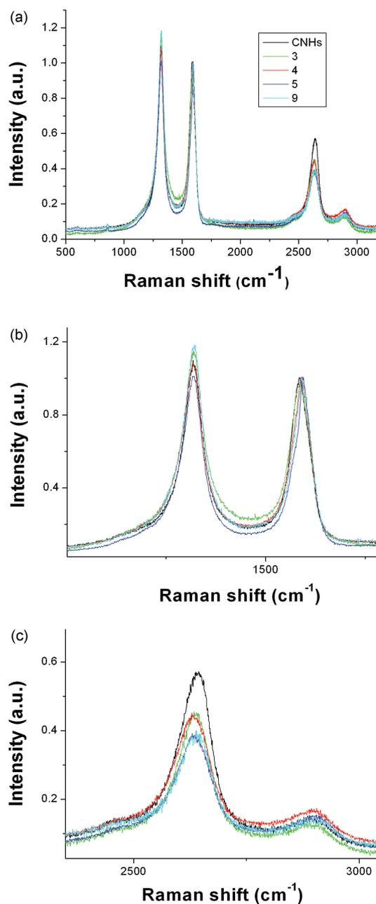
Fig. 3 (a) Raman spectra (633 nm) of pristine CNHs, *f*-CNHs 3, 4, 5 and 9, (b) detailed D-region, (c) detailed G' and D+D' region.
