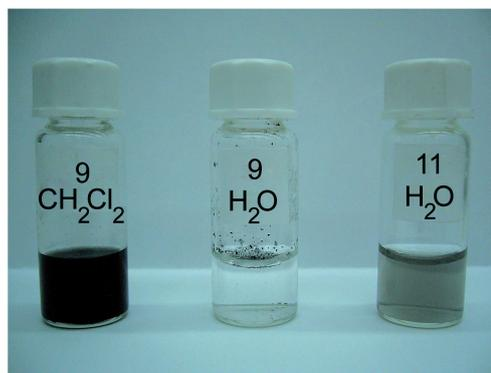
**Fig. 6** Solubility test: *f*-CNHs **9** (4.3 mg) were dispersed in 1 mL of CH<sub>2</sub>Cl<sub>2</sub> and 1 mL of H<sub>2</sub>O and the corresponding deprotected *f*-CNHs **11** (0.75 mg) were dispersed in 1 mL of H<sub>2</sub>O.
