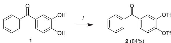
**Scheme 1** Synthesis of **2**. *Reagents and conditions:* *i*, CH<sub>2</sub>Cl<sub>2</sub>, **1** (1.0 equiv), –78 °C, pyridine (4.0 equiv), Tf<sub>2</sub>O (2.4 equiv), –78 to 0 °C, 4 h.
