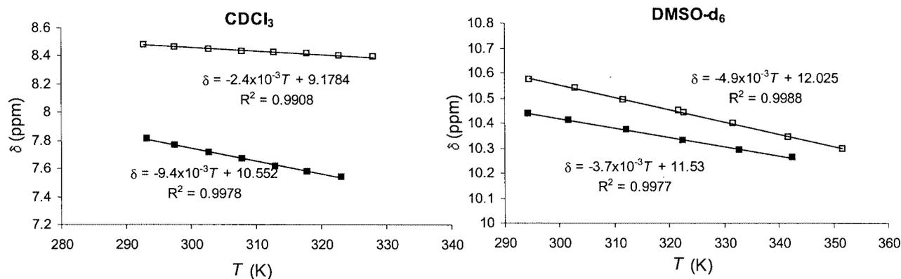
Figure 1. Temperature dependence of  $^1\text{H}$  NMR chemical shifts for the amido protons of **3-Z** (□) and **3-E** (■) in  $\text{CDCl}_3$  and  $[\text{D}_6]\text{DMSO}$
