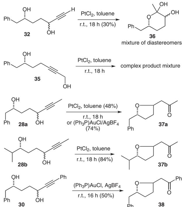
**Scheme 5** Reactions of alkyne diols **32** and **35** with  $\text{PtCl}_2$ . Cyclization of the alkyne diols **28a**, **28b**, and **30** to the tetrahydrofurans **37a**, **37b**, and **38**, respectively, via metal-induced Meyer–Schuster rearrangement and oxa-Michael addition
