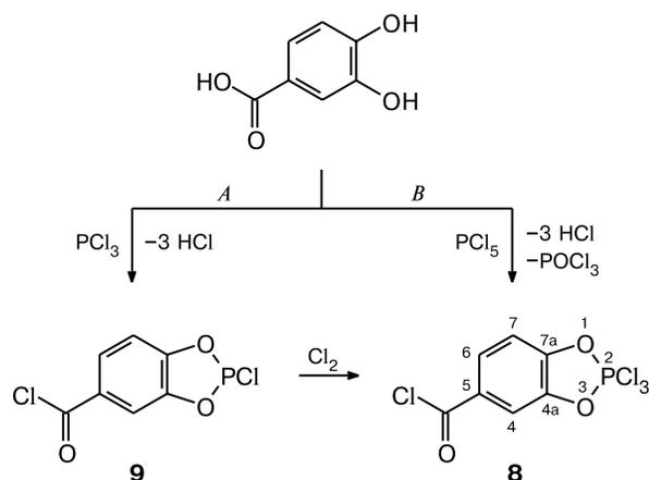
uct **8** in moderate yields. The reactions were accompanied by chlorination of the carboxy group to form the chlorocarbonyl group. Since the molecule cannot contain simultaneously the free carboxy group and the phosphorane fragment with three P—Cl bonds,<sup>6</sup> the reaction was carried out in the presence of a two-fold excess of  $PCl_3$  or  $PCl_5$ .
