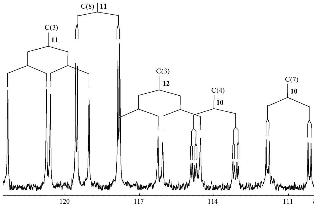
**Fig. 1.** Fragment of the high-field region of the  $^{13}\text{C}$  NMR spectrum of a mixture of compounds **10**–**12** prepared by the reaction of benzophosphole **8** with phenylacetylene (before heating).
