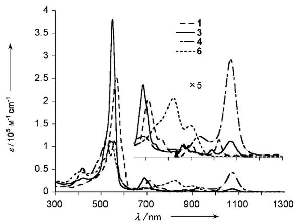
**Figure 2.** UV/Vis absorption spectra of **1**, **3**, **4**, and **6** in  $\text{CH}_2\text{Cl}_2$ .
