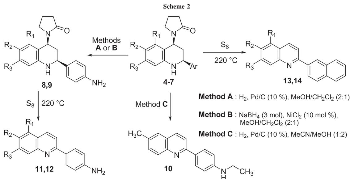
ring aromatization reaction with pyrrolidine fragment elimination, (2) nitro group reduction into amine function, (3) N-ethylation of amine group to give *N*-ethylamino derivative **10** (Scheme 2). Its quinoline structure was strongly confirmed by <sup>1</sup>H-, <sup>13</sup>C-NMR spectra and 2D NMR spectroscopy.
