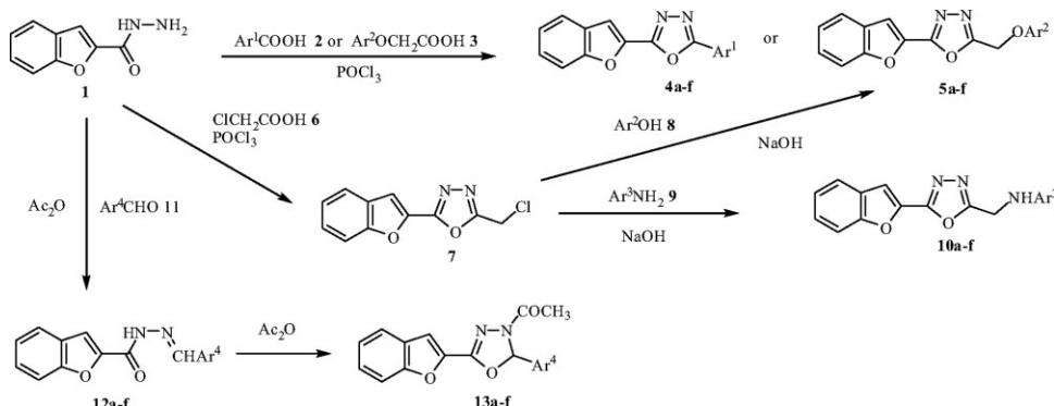
**1** with aryloxyacetic acids (**3a-f**) need catalytic amounts of pyridine in reflux  $\text{POCl}_3$  and longer time (8 h) to give the corresponding 1,3,4-oxadiazoles (**5a-f**) in higher yields (method A) (entries 7–12, Table 1).
