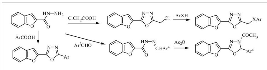
In this study, the synthesis of series of 2-benzo[*b*]furan-substituted 1,3,4-oxadiazole derivatives using readily available 2-benzo[*b*]furan carboxylic acid hydrazide as starting material has been investigated.
