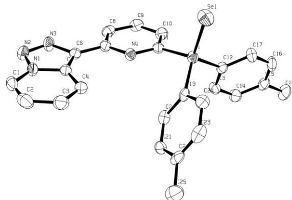
**Fig. 3** Solid-state molecular structure of **3e** (**B**). Hydrogen atoms are omitted for clarity. For details see ESI.†
