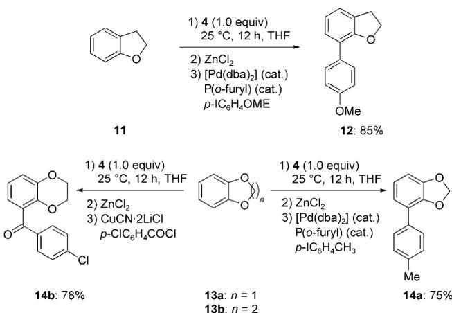
**Scheme 3.** Almination of substrates with annelated oxygen-containing rings and subsequent transmetalation with  $\text{ZnCl}_2$ , followed by copper-mediated acylation or palladium-catalyzed cross-coupling.
