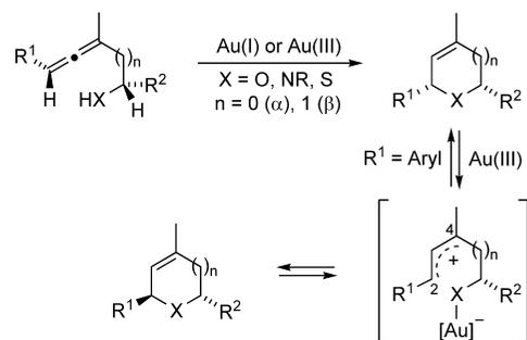
In contrast to alkyl-substituted allenes, substrates bearing phenyl or electron-rich aryl substituents  $\text{R}^1$  undergo epimerization when treated with gold(I) or gold(III) precatalysts in
